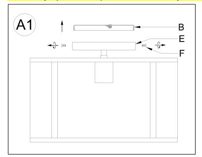
Separate the Mounting Plate (B) from the Canopy (E) by removing the 2 Canopy Screws (F). Do not discard the Canopy Screws (F) as these will be used later.
