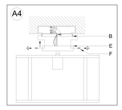
With the help of another people to hold the weight of the light fixture, position the Canopy (E) over the Mounting Plate (B), aligning the 2 holes on the Canopy (E) with the 2 holes from the Mounting Plate (B). Insert the 2 Canopy Screws (F) and tighten to secure the Canopy (E) in place.
