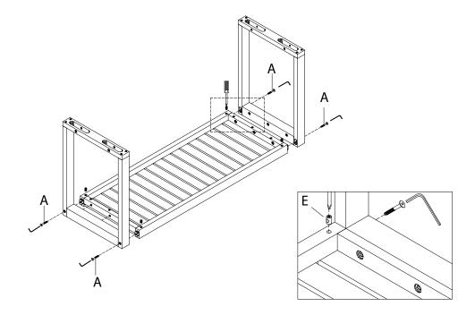
2. Insert 6 bolts (C) into the holes in the table top as shown. Tighten with allen key.
