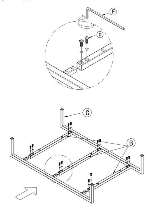
2. Put the case (A) upside down on the soft surface and attach the metal base as the illustration below, Tighten 6 Bolts (E) by Allen Key (F).
