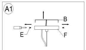
Separate the Mounting Plate (B) from Canopy (F) by removing the Canopy Screws (E). Do not discard the Canopy Screws (E) as these will be used later.
