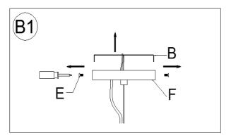
Separate the Mounting Plate (B) from Canopy (F) by removing the Canopy Screws (E). Do not discard the Canopy Screws (E) as these will be used later.
