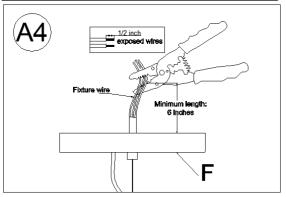
If needed, cut off the extra power cord length on the 3 wire cords so that they all are at least 6 inches (152.4 mm) long within the outlet junction box (J-box).
