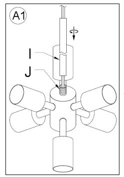
Insert the fixture 2 wire power cord and bare copper ground wire through the 6 in. Tube (I), and attach bottom end of the 6 in. Tube (I) onto the Threaded Pipe (J) and turning in a clockwise direction until tight.
