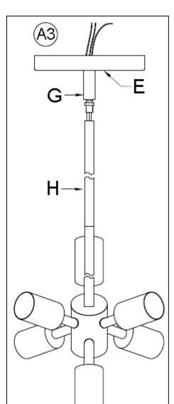
Use the additional 12 in. Tubes (H) as needed to adjust the fixture's suspension length by following the similar procedure as outlined in step 2.
