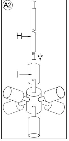
If you would like to use only one 12 in. Tube (H), then thread the 2 wire power cord and bare copper ground wire through the 12 in. Tube (H), making sure the tube nipple joint end is downward as shown in diagram. Attach the bottom end of 12 in. Tube (H) onto the top end of 6 in. Tube (I) and rotate clockwise until tight.
