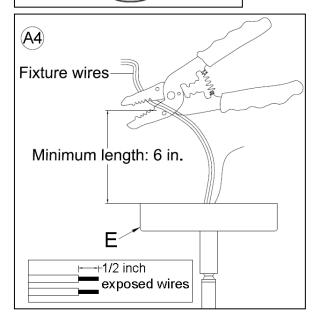
If needed, cut off the extra power cord length on the 2 wire cords and bare ground wire so that they all are at least 6 inches (152.4 mm) long within the outlet junction box (J-box).
