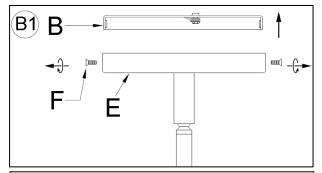
Separate the Mounting Plate (B) from the Canopy (E) by removing the 2 Canopy Screws (F). Do not discard the Canopy Screws (F) as these will be used later.
