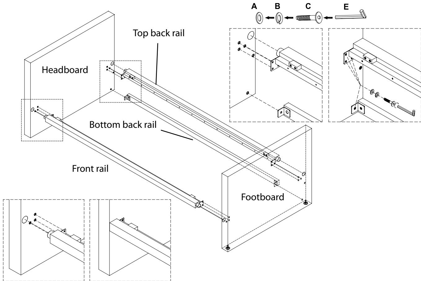
2. Secure the wooden corner blocks to headboard/footboard and top back rail using bolts (D) and tighten with the allen key (E).
