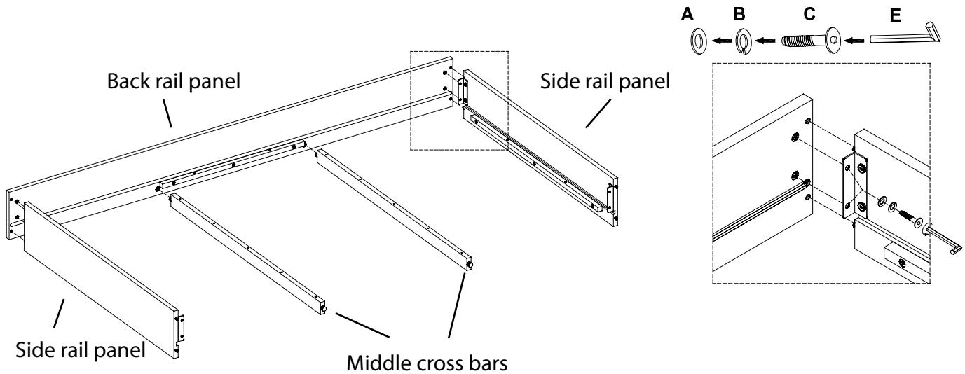
6. Assemble bottom panels to side and back rail panel by inserting into groove of the panel as shown below.
