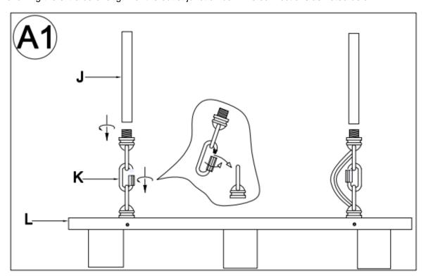
Attach the Shade Canopy (L) loops onto the bottom loops of the Tubes (H) using the Chain Quick Links (K). Close each Chain Quick Link (K) by turning the nut onto the threaded end of the Chain Quick Link (K) until tight
