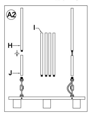
If you would like to add only a length of 6 inches, then thread the 2 wire power cord and bare copper ground wire through a 6 in. Tube (J), making sure the tube nipple joint end is downward. Attach the 12 in. Tube (H) onto the top of the Tube (J) and rotate the 12in. Tube (H) clockwise until secure. Then, attach the other 12 in. Tube (H) onto the other Tube (J) and rotate the 12 in. Tube (H) clockwise until secure.
