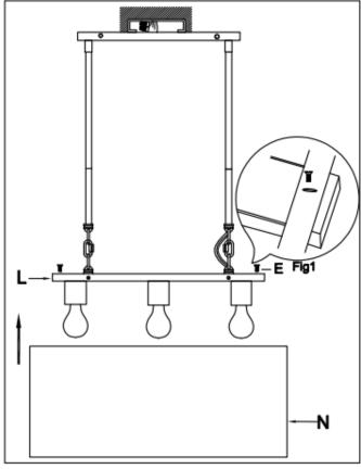
Attach the Shade (N) (not included) onto the Shade Canopy (L) using the Shade Screws (E) and tighten with a screwdriver until secure.
