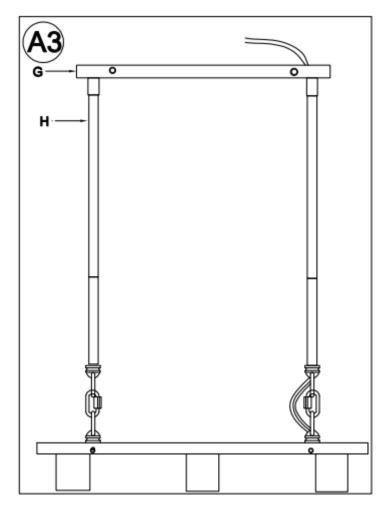
Thread the fixture's 2 wire power cord and bare copper ground wire through the one bottom tube opening in the Canopy (G). Then, attach the two 12 in. Tubes (H) onto the bottom Canopy (G) by rotating each tube clockwise until secure.
