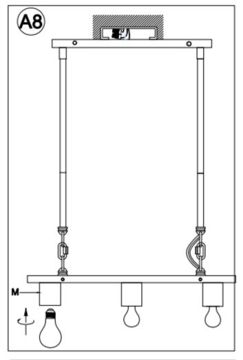
Insert there (3) specified light bulbs into the Sockets (M). DO NOT EXCEED THE SPECIFIED WATTAGE
