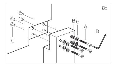
Attaching the headboard to beframe for mattress only: Align hardware as shown and tighten.
