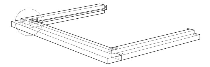
\*NOTE: Do not fully tighten all bolts until all parts are fully assembled.
