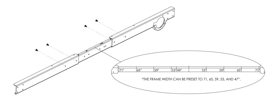
Mount motor unit on stretcher bar using three M5 screws.
