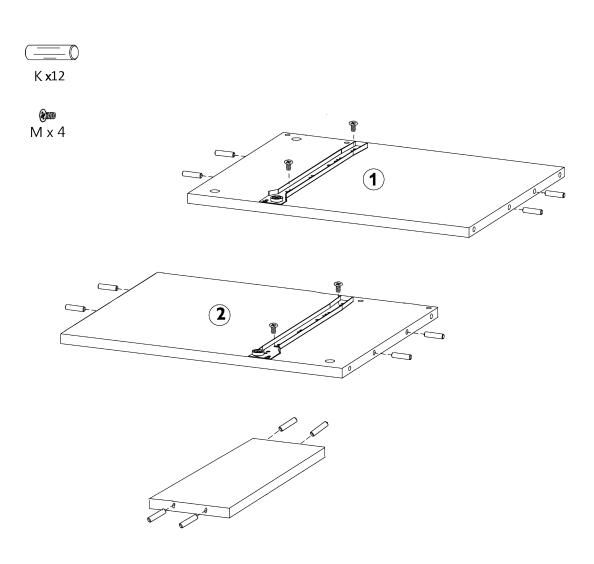
7. Insert cam screws (B) into top panel as shown.
