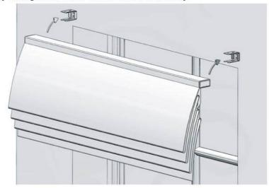
**Step 7:** Once the headrail is properly centered within the brackets, use a screwdriver and a provided short screw to secure the mounted headrail to each end bracket (securement to the third central bracket, if there is one, is not necessary).
