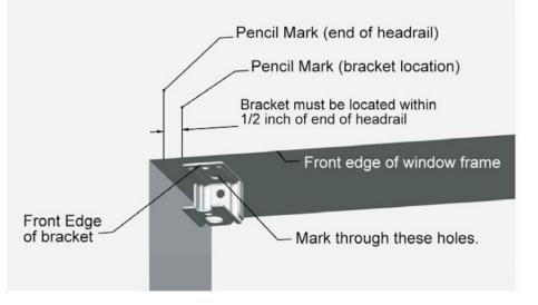
**Step 3:** To prevent any wood from splitting when screws are secure therein, we recommend that pilot holes be drilled at the marked locations for the brackets. Use a power drill and a 1/8 inch drill bit to drill a hole at each mark that is about 1 in deep.
