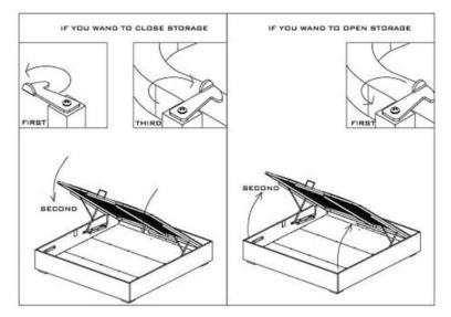
Make sure lock is enganged when mattress is not on metal frame to be sure that the metal frame does not raise unexpectedly.
